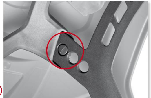
Push the adaptor button towards the outer shell. Now you can select one of the three ride heights by pushing the button in or out. Here, too, make sure to make the same adjustments on both sides!
