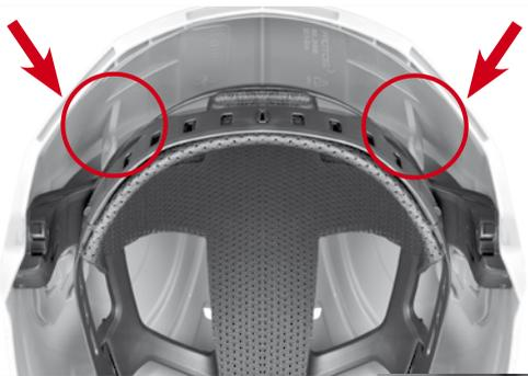
There are two more fasteners at the front of the chin strap (Fig. 6). Snap both of these into the sockets on both sides (circles). Lock them into place by pulling slightly, so that they point to the inside of the helmet (Fig. 11).
