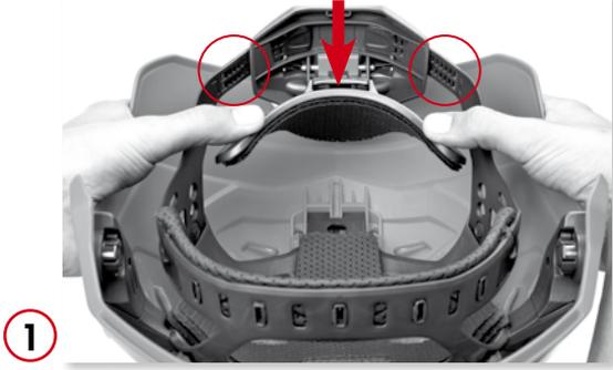
Push the neck **guard** towards the inside of the helmet until it snaps into place (with a slight click). In this position you can see the right and left adjustment **straps** (see circle Fig. 3). Use these to adjust the Protos® Integral safety helmet to your head size.
